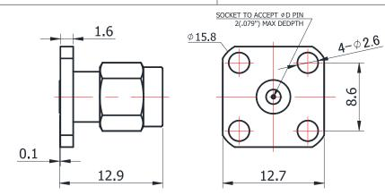
For glass-bead of 0.30mm pin diameter
